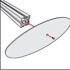
Base Plate & Extrusion Connection
