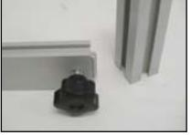
Detail F: Plastic Star Knobs are used to tighten locks where horizontal extrusions connect with vertical extrusions. Turn the knobs clockwise to tighten. Turn counterclockwise to loosen, but do not remove knob.
